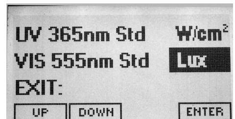
Press ENTER to return to left column, DOWN to highlight EXIT and ENTER again to access UNITS.
