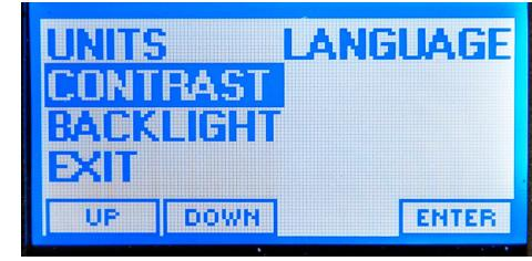
Press ENTER to access the next screen, where the default contrast level is 48, which gives the best display in most lighting environments. This level can be changed to range from 42 to 55 by pressing UP or DOWN. Press EXIT to save the setting and return to the previous screen. **NOTE:** Any changes to the contrast level will revert to default level when the AccuMAX is shut off.
