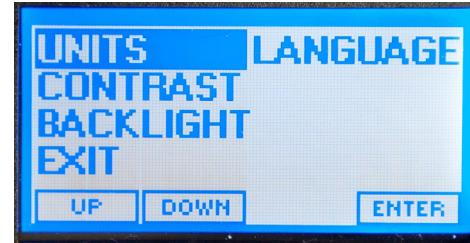
Press UP or DOWN to highlight the feature to be changed and ENTER to access the next screen, or highlight EXIT and press ENTER to return to OPERATION.
