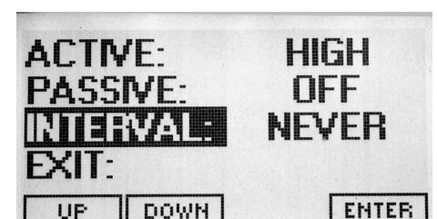
Press ENTER again to access the right column to set the length of time (60sec, 30sec, 10sec) between ACTIVE and PASSIVE operations.
