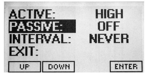
Press ENTER and then UP or DOWN to change the BACKLIGHT setting in the right column.
