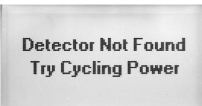
and will automatically shut off in 30 seconds. This same message is displayed if the detector is removed while the instrument is running. To remedy this situation, simply turn off the AccuMAX, plug in the detector, and turn the unit on. The instrument will then initialize itself automatically.
