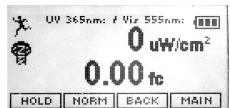
NOTE: The meter will immediately begin registering any subsequent changes in light level.
