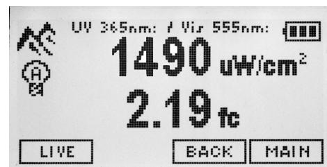
When in PEAK function, press LIVE to return to NORMAL mode, or press BACK to return to the previous HOLD screen, and press BACK again to return to NORMAL mode.
