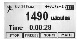
While integrating, press FREEZE to freeze and hold the displayed data. The snowflake icon will indicate that the display is static.
