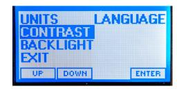
Press ENTER to access the next screen, where the default contrast level is 48, which gives the best display in most lighting environments.
