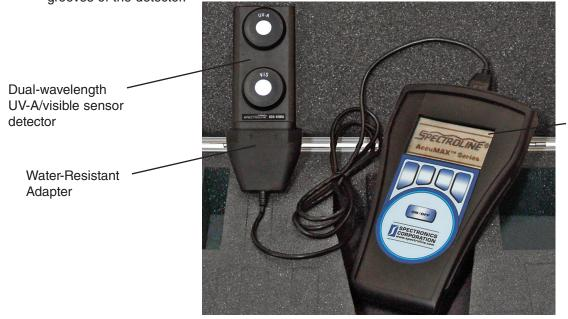
LCD window with numbers, units, modes and system status. Displays multiplexed data from UV-A/visible output.
