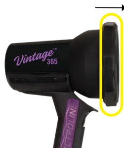
The glass filter will remain inside the protector. To remove the glass filter, peel around the edge of the rubber cover/filter holder and push the glass filter out. To replace or reinsert the glass filter into the rubber cover/filter holder, slide the glass filter into the channel of the rubber cover/filter holder. Manipulate the rubber cover around the filter. Ensure the glass filter is evenly seated.
