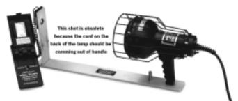
Avoid a "balancing act." Use the Spectroline Model VF-100 Spec-Stik™ MIL-STD verification fixture to calibrate your lamps at *exactly* 15 inches (38.1cm)!
