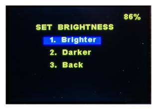
Press the **MENU** button until desired brightness level is attained. Press **BACK** to confirm and exit.
