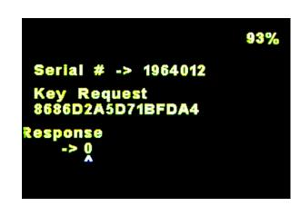
Zeroes will appear in the *Response* field each time the **MENU** button is pressed. The text "**Verify Bad**" will display (as shown below) and the device will then automatically exit the calibration screen, returning to the Main Menu by default.
